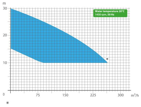
Range of capacity diagram. For best hydraulic performance we use adjusted pump housing and impeller design.
